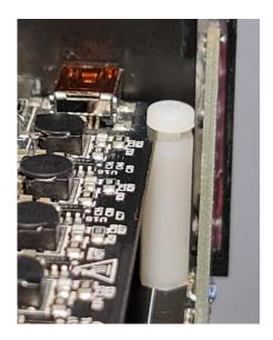
Use 2 of the nylon screws on the right-hand screw holes to affix the PCB to the expansion board. Check
