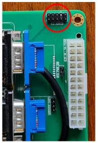
• Connect up your case USB header. Note that the Ultimate Expansion board has both USB2 and USB3 headers available. Only connect ONE of these at any time, as their data lines are connected.
