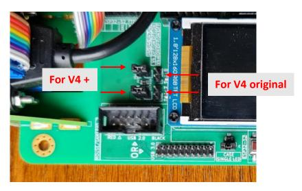
Select case LED type – Place a jumper ON for single case for power and HDD access, or leave jumper OFF (default) for separate case power and HDD front panel LEDs.
